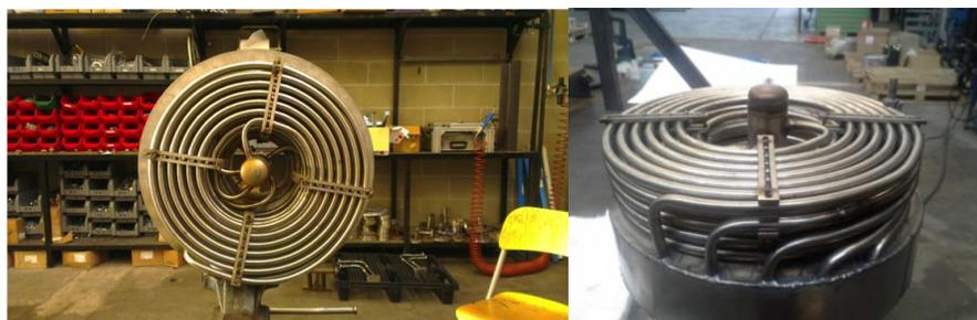
**Figure 3.**Picture of the spiral heat exchangers
