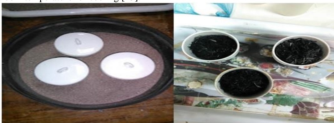
Figure 2: Crucible and steel container used for activated carbon.
