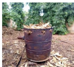
Photo 1: Loading corn stalks into the carbonizer
