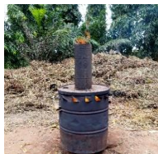
Photo 2: Carbonization of corn stalks in a low-oxygen environment
