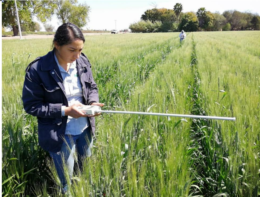
Figure 2. Taking readings of the leaf area index area using a linear ceptometer AccuPAR LP-80.
